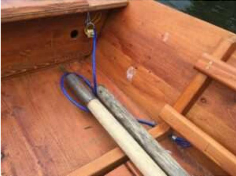
Pass the short front steel cable in the punt through the eyelet on the T-beam.
