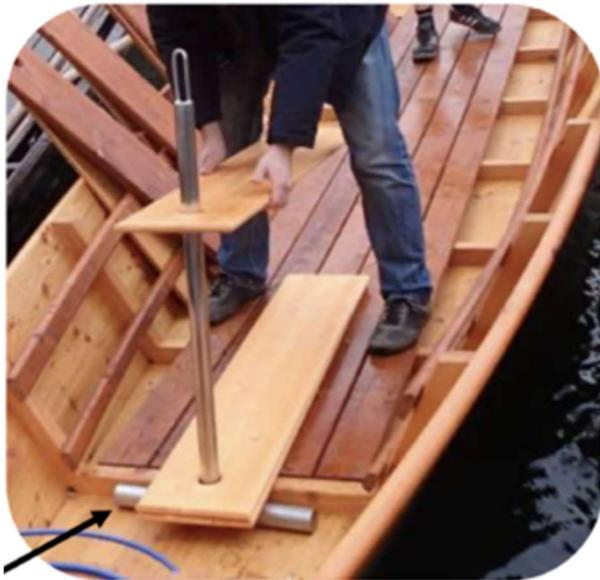
Start with the boards closest to the front of the barge (shore side, board nr. 8). Always stack one seat board and 2 backs, next seat board and 2 backs... Pay attention to the order and these "packs of 3".
