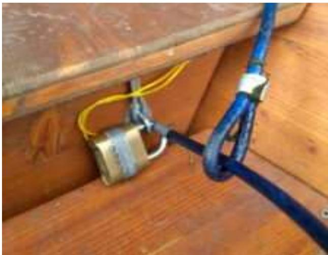
**Now both poles, all boards and both boxes should be connected or locked and a steel cable is pulled through the ring on the shore and a cloth rope is hooked. Check again if the padlocks are really closed.**
