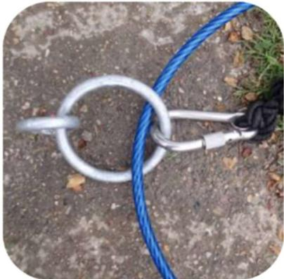
Put the steel cable from the board stack through the loop of the steel cable coming from the shore.
